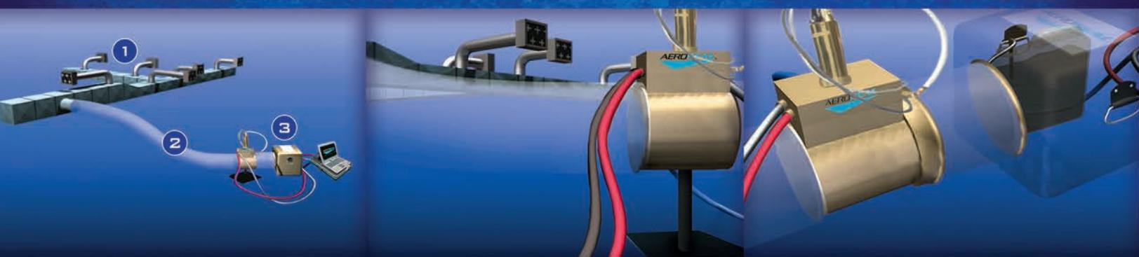
Once the Duct Leak Analysis is completed and approved, all supply and return grilles are temporarily sealed
